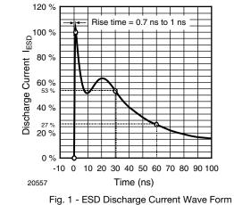
Fig. 1 - ESD Discharge Current Wave Forn acc. IEC 61000-4-2 (330 Ω/150 pF)
