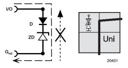
Another PN-diode "opens" the back path so that the protection device becomes bidirectional! Because the clamping voltage levels in forward and reverse directions are different, such a protection device has a **Bi**directional and **As**ymmetrical clamping behaviour (**BiAs**) just like a single Z-diode.
