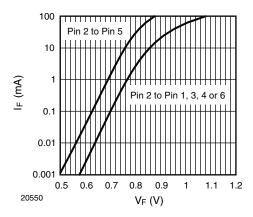
Fig. 4 - Typical Forward Current I<sub>F</sub> vs. Forward Voltage V<sub>F</sub>
