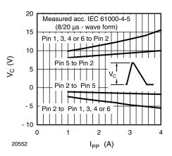
Fig. 6 - Typical Peak Clamping Voltage V\_C vs. Peak Pulse Current  $I_{\text{PP}}$
