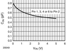
Fig. 3 - Typical Input Capacitance C\_{IN} at Pin 1, 3, 4, or 6 vs. Input Voltage  $V_{IN}$
